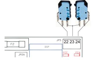
N.B. The LEDs that correspond to the limit switches are ON when the relative limit switch is not involved.
