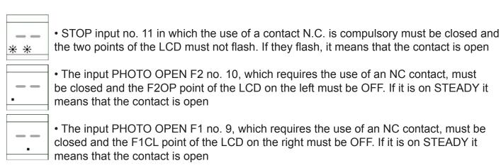
N.B. In normal use, the points of the LCD must not flash or be on steady. They flash or stay on if the corresponding safety is activated.
